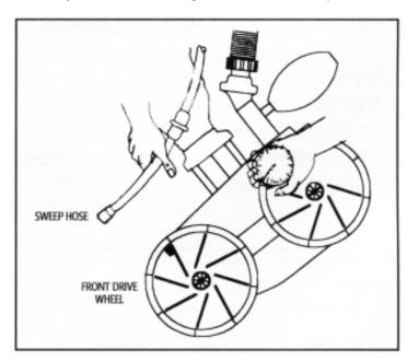
Mark the front drive Tire/Wheel with a marker, or use the Logo located on the side of tire as a marker to count the rotations of the wheel per minute.
